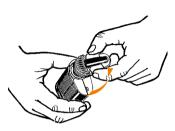
Removal of Cooling Unit (with Mouthpiece)
