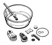
Manual cleaning of the disassembled Cooling Unit
